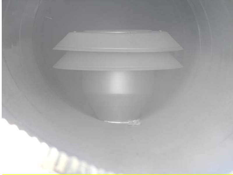
Figure 2-4. View of R&P PM 10 TEOM Sampling Head in Combined Sampling Duct, Barstow
