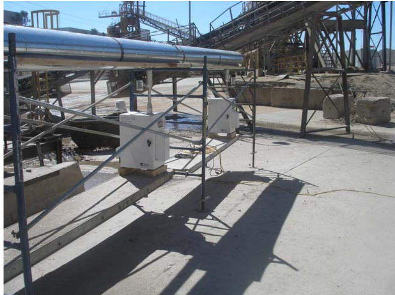
Figure 2-2. Side View of Combined Sampling Duct, Carroll Canyon (FRM 2000 PM 4 Monitor Left, PM 10 TEOM Monitor Right)
